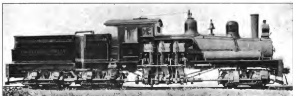
Fig. 130. Twelve-Wheel Shay Geared Locomotive. Built by the Lima Locomotive & Machine Co. for the Tioga Lumber Co.
